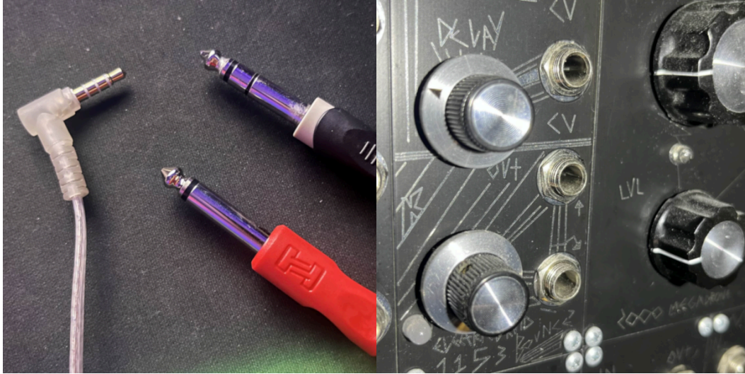
Figure 3.X Male & Female 1/4" audio connectors (with male 3.5mm for reference). Image Source: Author
